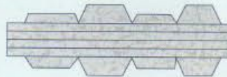
"FULLY WRAPPED" SECTION, DRIVE CLEAT ON SIDES ONE AND THREE, OR TWO AND FOUR, PROGRAMMERS CHOICE.
