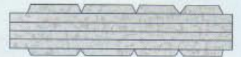
THE PROGRAMMER CAN PUT DRIVE CLEATS ON ALL 4 SIDES OF THE DUCT IF REQUIRED.
