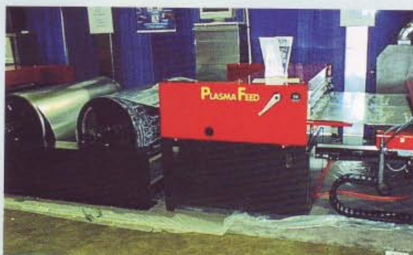
PLASMA FEEDER Feeds plasma table with coiled flat sheet from 2 or 4 coil holders. Max gauge 16 Gauge mild steel. Beading available at no extra cost. Hydraulically operated. Optional power fed coil holders.
