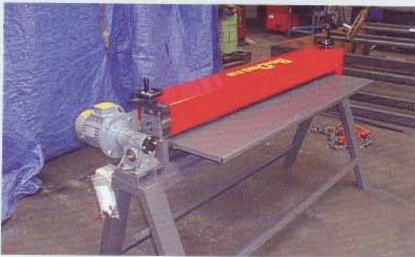
BEADER 518 Freestanding Beading Machine. 56" 1500mm wide 18 Gauge Max Mild Steel
